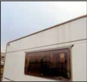
Black streaks may indicate mastic breakdown
